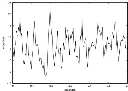
Fig. 1: Raw example of the electrical activity of the brain captured on a surface EEG (abscissa in s, ordinate in  $\mu V$ ).
